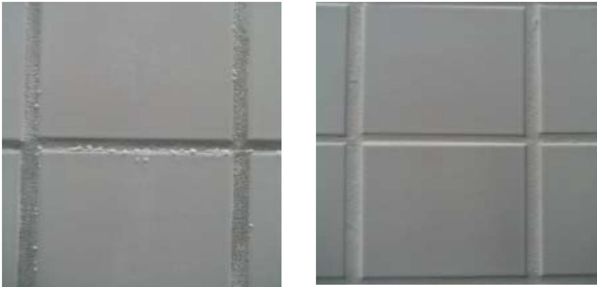
*Image 10: Joint grout surfaces after weathering.
