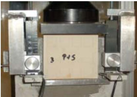
*Image 1: Device to determine the absolute deflection of a tile from static conditions*
